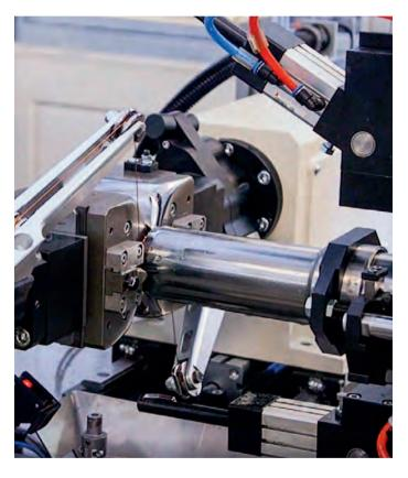
As a basic technology for the production of electric motors, winding technology is indispensable for a comprehensive automation offer. Our specialists have decades of experience in this field and produce sophisticated winding machines. These robust systems are integrated into our BBS production lines or offered as a stand-alone solution.
